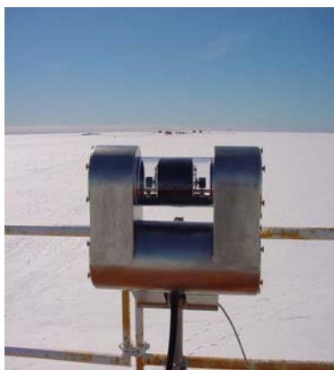
Figure 6.3.1-11. The new multi-axis DOAS telescope at the Neumayer-Station, Antarctica.
