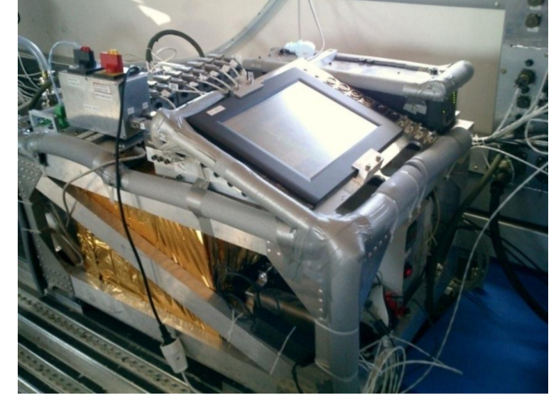
The IUP Bremen imaging DOAS instrument rack in the Polar-5 aircraft:
