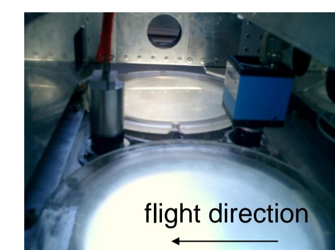
Nadir viewing ports: spectrometer objective (left) & picture camera (right)
