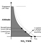
Model VMR at the surface:  $\chi_s$ Shaded area: VCD Scaling factor:  $VCD/\gamma$ . Observed VMR at the surface:  $\chi_{abs}$ Scaled VCD:  $\chi_{obs} \times (VCD/\chi_s)$
