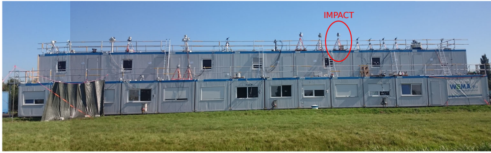
Figure 8.3: Set-up on roofs of containers: Ground level: 1D MAX-DOAS; Top level: 2D MAX-DOAS.
