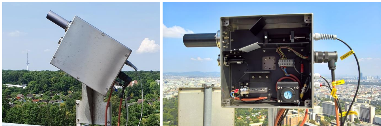
Figure 3. The MAX-DOAS telescope units as installed on the roof of the IUP Bremen. The closed telescope box is looking above horizon (left panel) and the inside of the telescope box (right panel).
