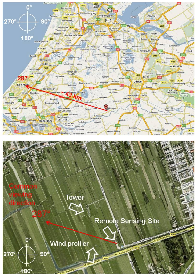
Figure 5.1: CINDI overview maps. Top: The measurement site is located between Utrecht and Rotterdam. The MAX-DOAS viewing direction ( 287^\circ from North) is indicated by a red arrow. The length of the arrow is 43 km, which is the horizontal distance inside a boundary layer of 1.5 km height under the condition of 2^\circ elevation angle. Bottom: Aerial picture of the measurement site. The instruments were installed predominantly at the remote sensing site (RSS), but also at the tower and the wind profiler (WP). The in situ instruments were installed in different altitudes at the tower. Source: Google maps ( http://maps.google.de ).
