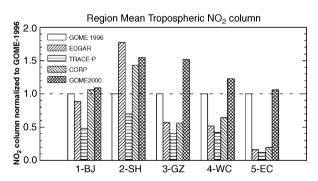
Fig. 6. Normalized tropospheric  $NO_2$  columns for the regions BJ, SH, GZ, WC and EC that are defined in Fig. 5. The mean model  $NO_2$  columns for emissions inventories EDGAR, TRACE-P and CORP and the mean GOME  $NO_2$  column for the year 2000 are scaled to the mean GOME  $NO_2$  column for 1996 in the same region.
